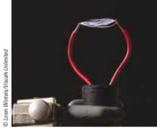
Figure 26.16 Dielectric breakdown in air. Sparks are produced when the high voltage between the wires causes the electric field to exceed the dielectric strength of air.
