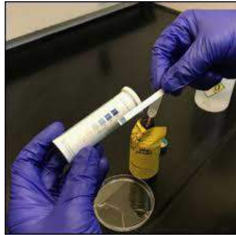
XploSens PS - Color Calibration (ppm with respect to aqueous hydrogen peroxide)
