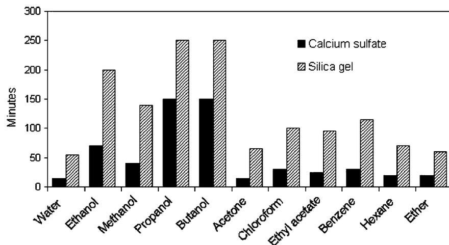
**Fig. 1.** Comparison of time taken by various solvents in developing TLC plates coated with calcium sulfate or silica gel
