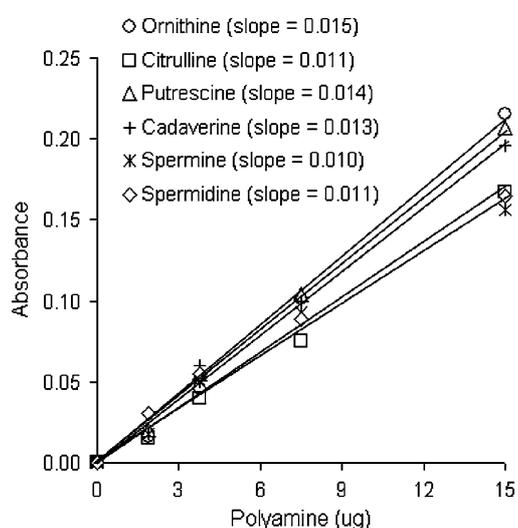
**Fig. 4.** Standard curves and their respective slopes for various polyamines
