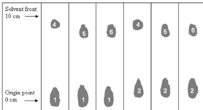
**Fig. 2.** Separation of ornithine (1) and citrulline (2) from cadaverine (4), spermine (5) and spermidine (6) on  $\text{CaSO}_4$  coatings using methanol as mobile phase
