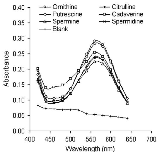
**Fig. 3.** Absorption spectra of various polyamines compared to blank
