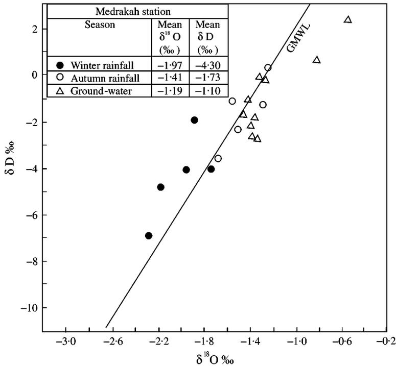
**Figure 7.** Deuterium-oxygen-18 relation in the ground-water of Wadi Ghiran basin.
