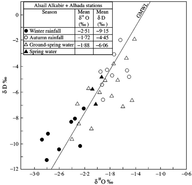
**Figure 6.** Deuterium-oxygen-18 relation in the ground-water and springs of Wadi Fatimah basin.
