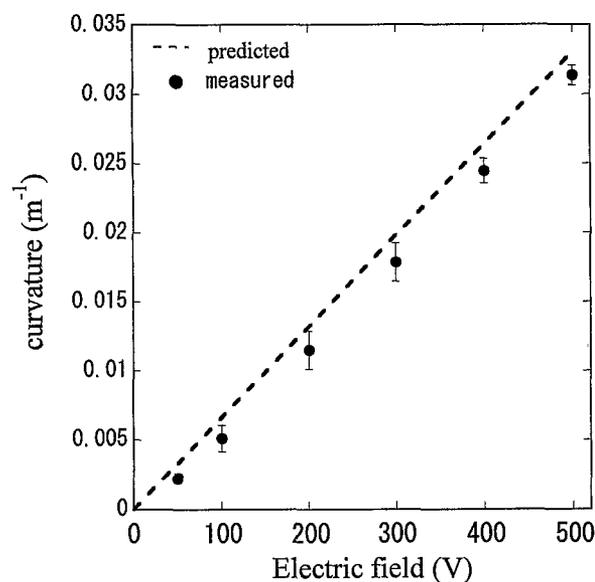
**Fig. 8.** Electric-field-induced curvature of the porosity-graded PZT beam-shaped actuator as a function of applied voltage.
