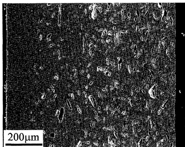
**Fig. 6.** SEM micrograph of the fabricated PZT sample with a linear porosity gradient.
