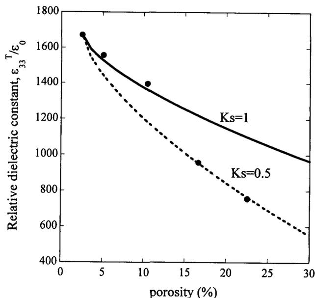
**Fig. 5.** Relative dielectric constants of PZT ceramics as a function of bulk porosity. The lines are the predicted values from Eq. (1) for two typical shapes of pores.
