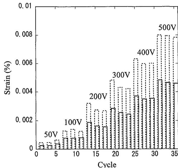
**Fig. 7.** Measured strains on the two sides (dotted lines: dense side; solid lines: porous side) of the FGM sample for different applied voltages from 50 to 500 V. Each voltage was repeated three times.
