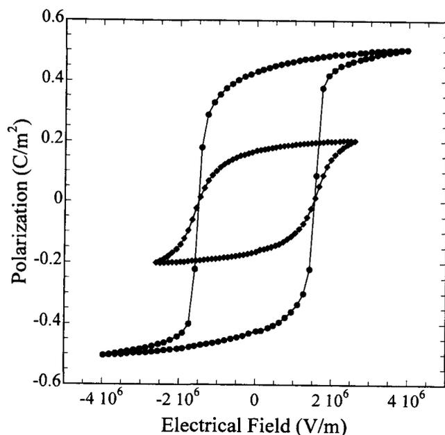
**Fig. 4.** Polarization–field hysteresis loops of 97.47% dense PZT (circles) and 83.38% dense PZT (diamonds) ceramics.
