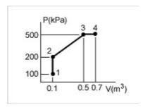
11- Air is compressed in an insulated piston-cylinder device. Using constant specific heats, ( $C_p$ =1.05 kJ/kg K, R=0.287 kJ/kg K). The amount of work required to compress this air from 100 kPa, 27°C to 2 MPa, 706°C is:
