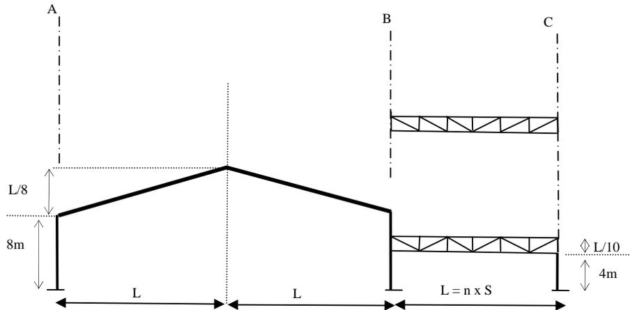
The main structural system of an industrial structure is composed of a steel frame between axis A and B, and a roof truss between axis B and C. The roof truss can have two different configurations as shown, with a span equal to  $L = n \times S$ , where  $n$ , is the number of truss panels and  $S$ , is the width of each panel. The clear height of the roof truss is 4m, while that of the steel frame is 8m. The main structural system is repeated with 8 equal spacing each equal to B.
