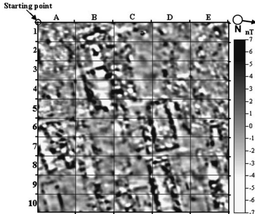
Figure 4. Magnetic image of the study area at Saqqara after application of the processing functions of the Geoplot program.
