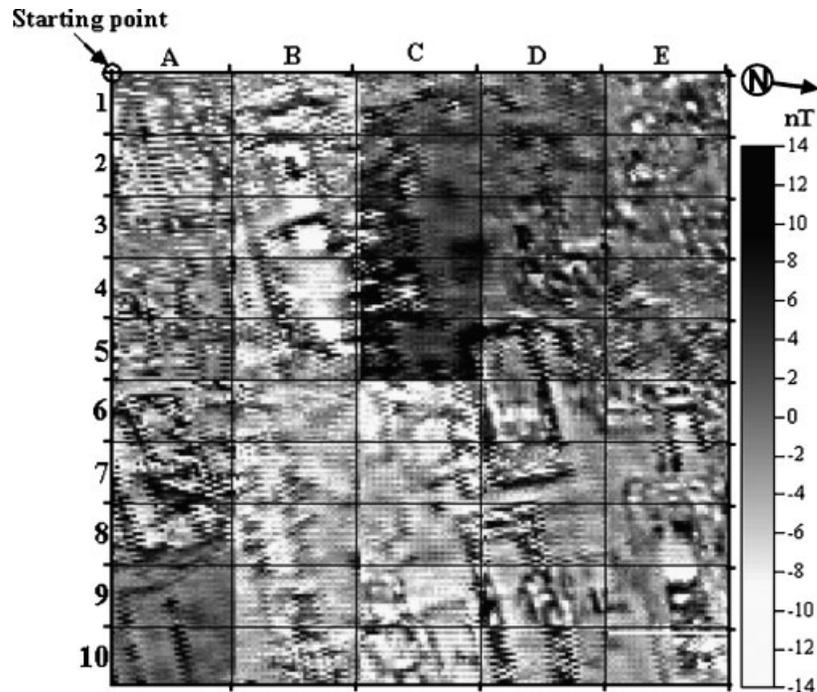
Figure 3. Magnetic image showing the raw data of the study area at Saqqara.
