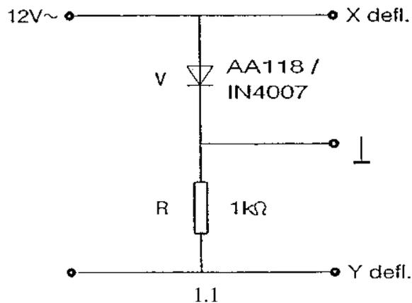
1. Assemble the circuit as shown in fig. 1.1 and apply an a.c. sinusoidal voltage  $V = 12\text{ V}$ ,  $f = 50\text{ Hz}$ .
