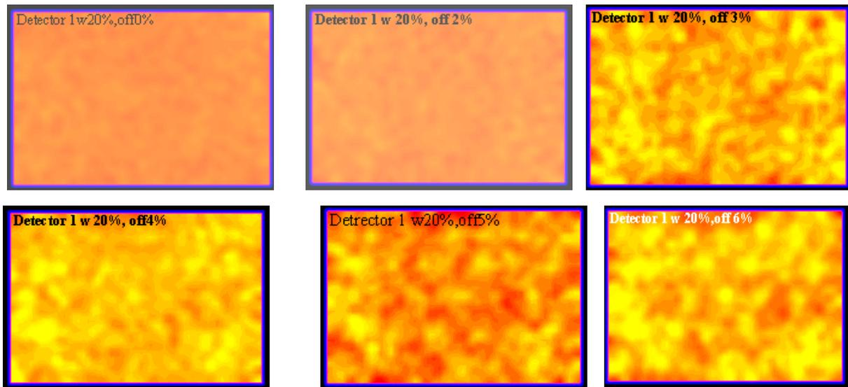
**Fig. 7** represents the flood images for different off-peak percentage at window width of 20%.
