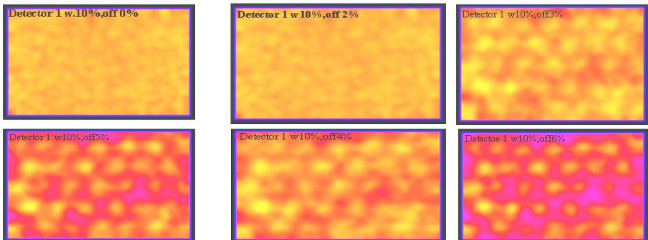
Fig. 5 represents the flood images for different off-peak percentage at window width of 10%.
