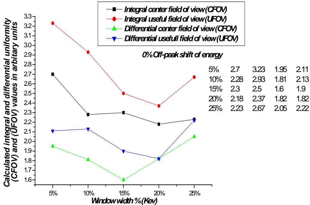
Fig. 8 represents the calculated integral and differential uniformity (CFOV) and (UFOV) values in arbitrary units versus Window width % in KeV at 0% off-peak shift of energy.
