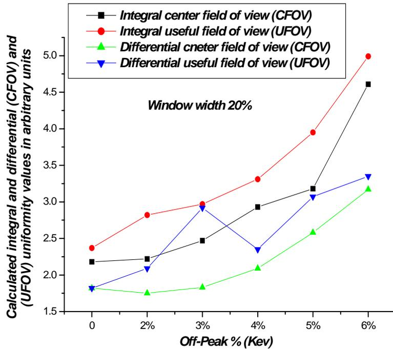
Fig. 4 represents the calculated integral and differential uniformity (CFOV) and (UFOV) values in arbitrary units versus Off-peak% in KeV at window width 20%.
