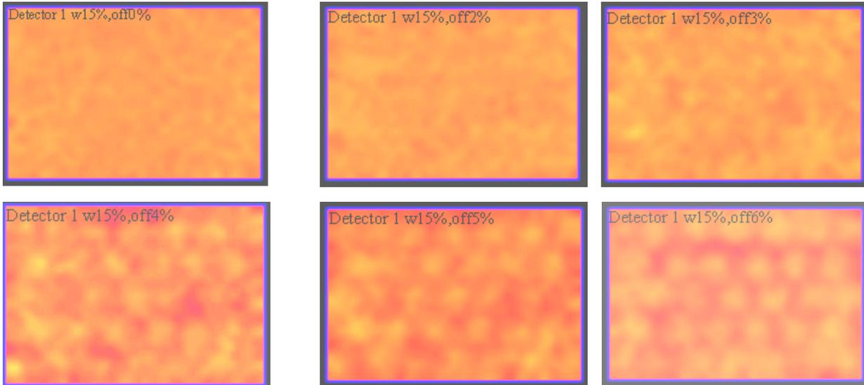
**Fig. 6** represents the flood images for different off-peak percentage at window width of 15%.
