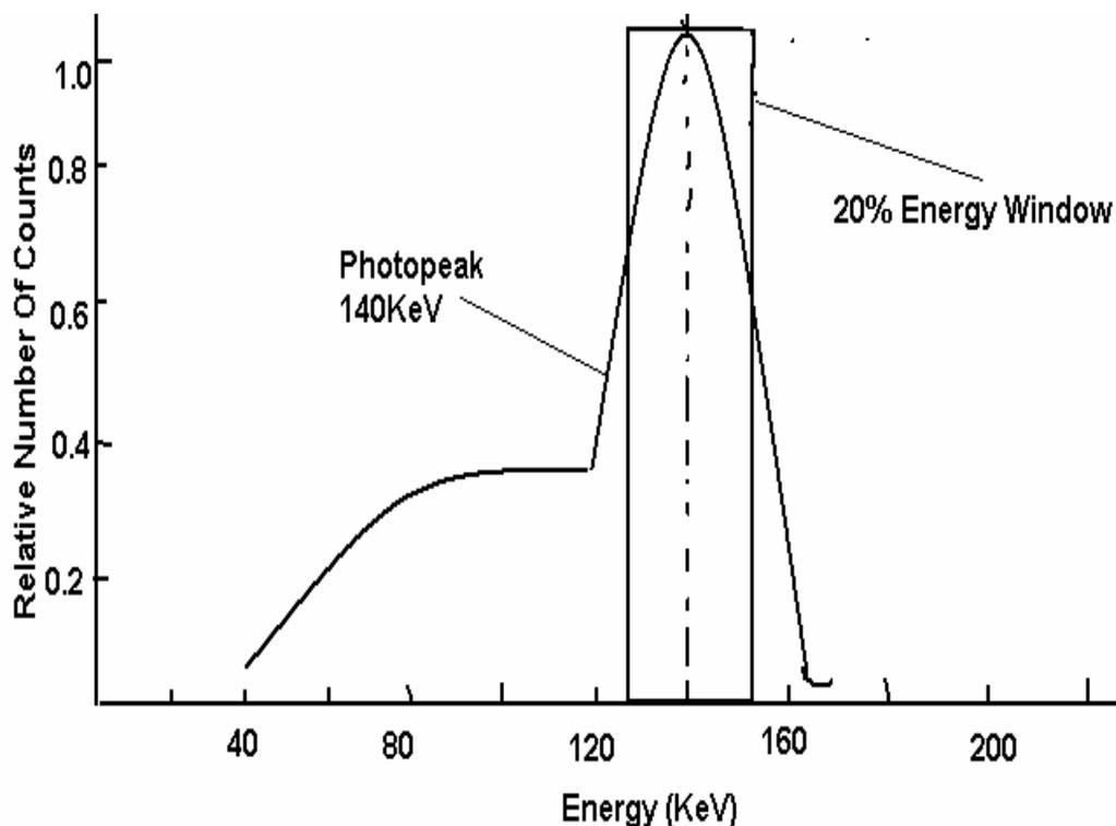
**Fig. 1 A photo-peak of Tc-99m at 140 keV and window width 20%**
