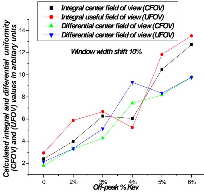
Fig. 2 represents the calculated integral and differential uniformity (CFOV) and (UFOV) values in arbitrary units versus Off-peak% in KeV at window width shift 10%.
