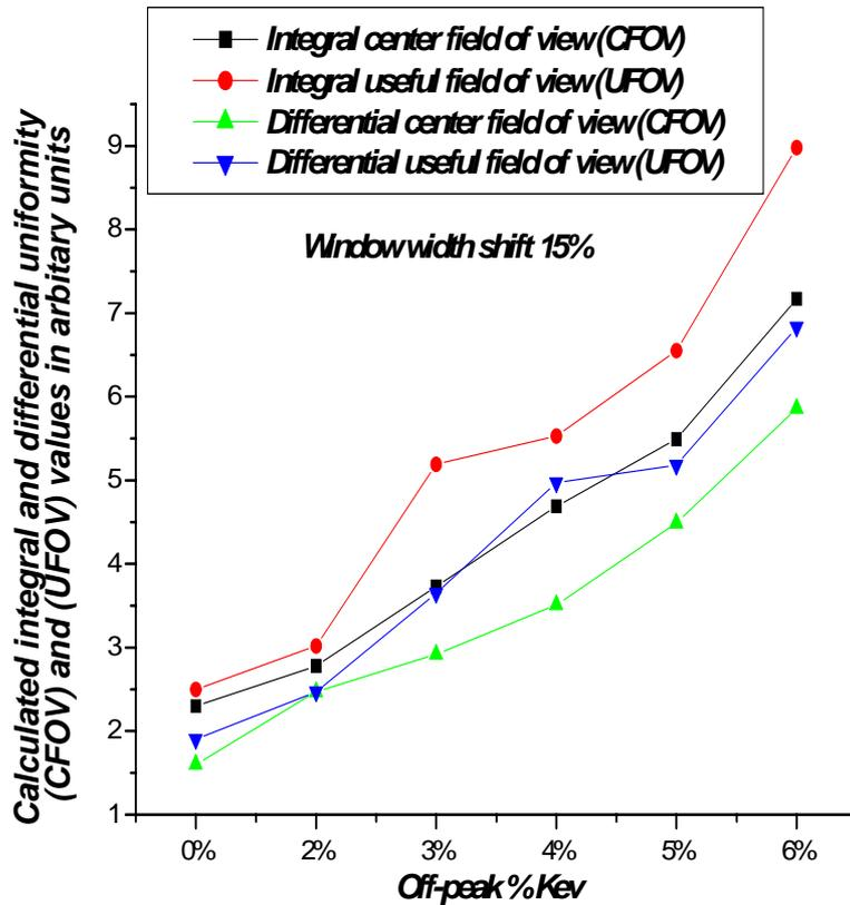
Fig. 3 represents the calculated integral and differential uniformity (CFOV) and (UFOV) values in arbitrary units versus Off-peak% in KeV at window width shift 15%.
