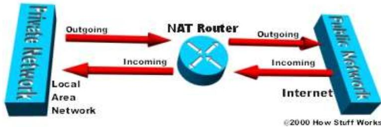
This is where NAT (RFC 1631 ) comes to the rescue. Basically, Network Address Translation allows a single device, such as a router, to act as agent between the Internet (or "public network") and a local (or "private") network. This means that only a single unique IP address is required to represent an entire group of computers to anything outside their network.
