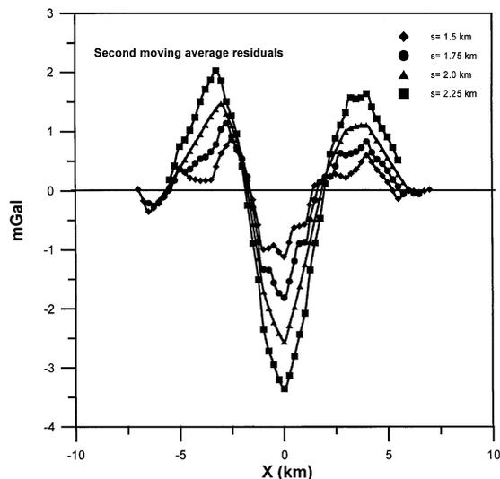
FIG. 8. Second moving average residual gravity anomalies on line AA' of the Humble dome for  $s = 1.5, 1.75, 2,$  and  $2.25$  km.
