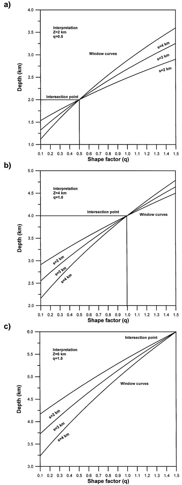
FIG. 3. Family of window curves of  $Z$  as a function of  $q$  for  $s = 2, 3,$  and  $4$  km using the present approach as obtained from gravity anomalies (a)  $\Delta g_1$  for  $q = 0.5$  and  $Z = 2$  km; (b)  $\Delta g_2$  for  $q = 1.0$  and  $Z = 4$  km; and (c)  $\Delta g_3$  for  $q = 1.5$  and  $z = 6$  km.
