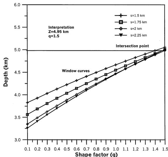
FIG. 9. Family of window curves of  $Z$  as a function of  $q$  for  $s = 1.5, 1.75, 2,$  and  $2.25$  km as obtained from the Humble gravity anomaly profile using our approach. Estimates of  $q$  and  $Z$  are, respectively, 1.5 and 4.95 km.
