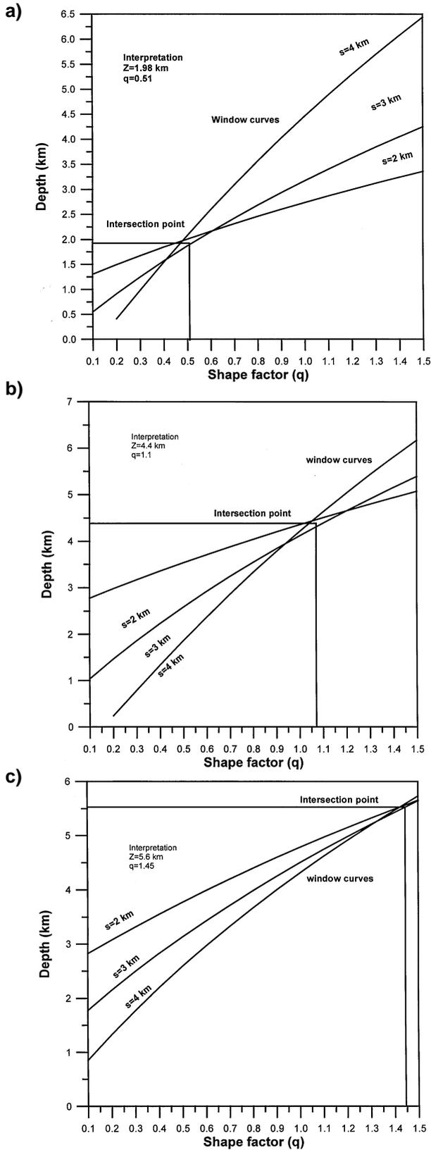
FIG. 5. Family of window curves of Z as a function of q for s = 2, 3, and 4 km after adding 10% random errors to the data using the present approach as obtained from (a)  $\Delta g_1$  for  $q = 0.51$  and  $z = 1.98$  km, (b)  $\Delta g_2$  for  $q = 1.1$  and  $z = 4.4$  km, and (c)  $\Delta g_3$  for  $q = 1.45$  and  $z = 5.6$  km.
