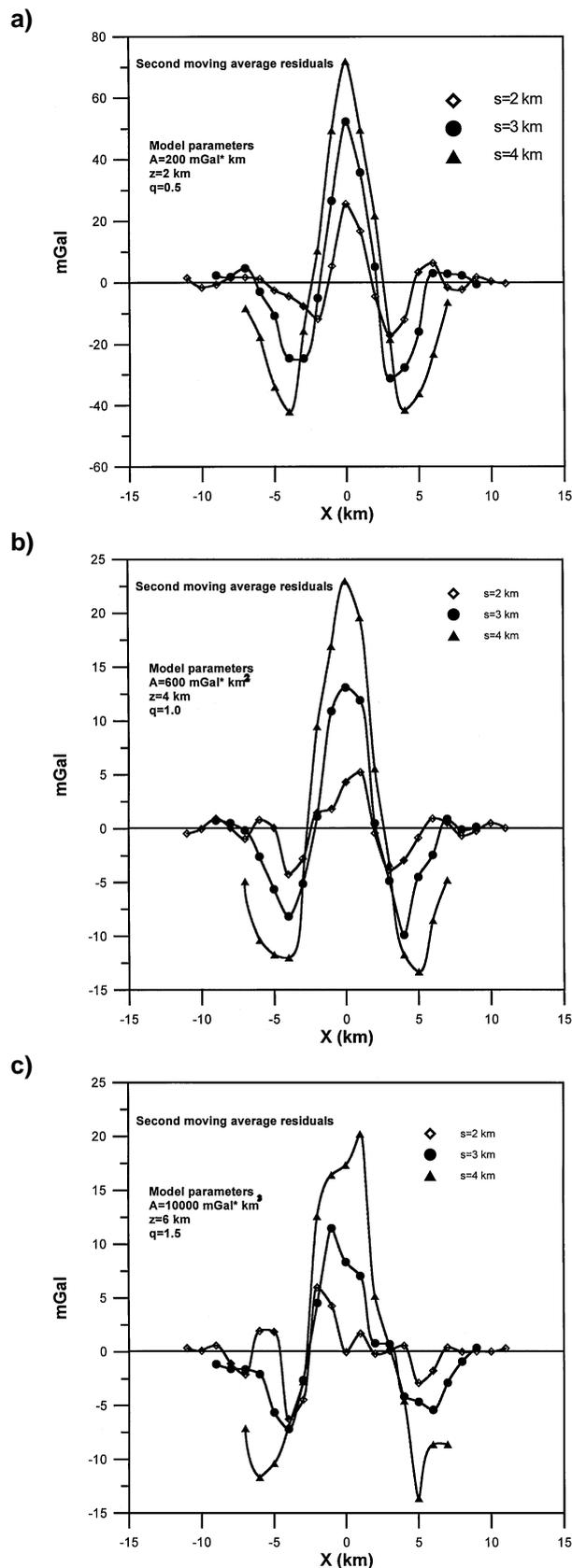
FIG. 4. Second moving average residual gravity anomalies for  $s = 2, 3,$  and  $4$  km after adding 10% random errors to the data as obtained from (a)  $\Delta g_1$ , (b)  $\Delta g_2$ , and (c)  $\Delta g_3$ .
