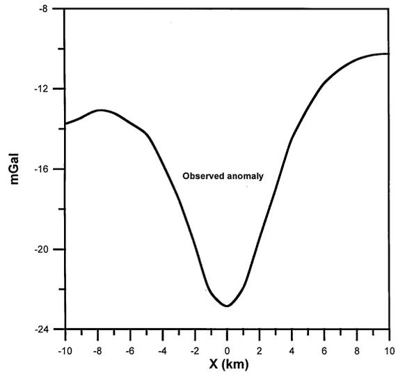
FIG. 7. Observed gravity profile on line AA' of the Humble dome near Houston.
