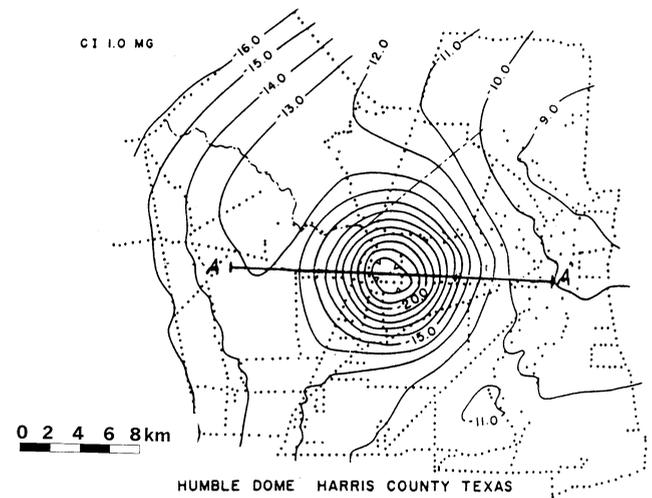
FIG. 6. Bouguer gravity map, Humble salt dome, Harris County, Texas (Nettleton, 1962). Computations are made along profile AA'.
