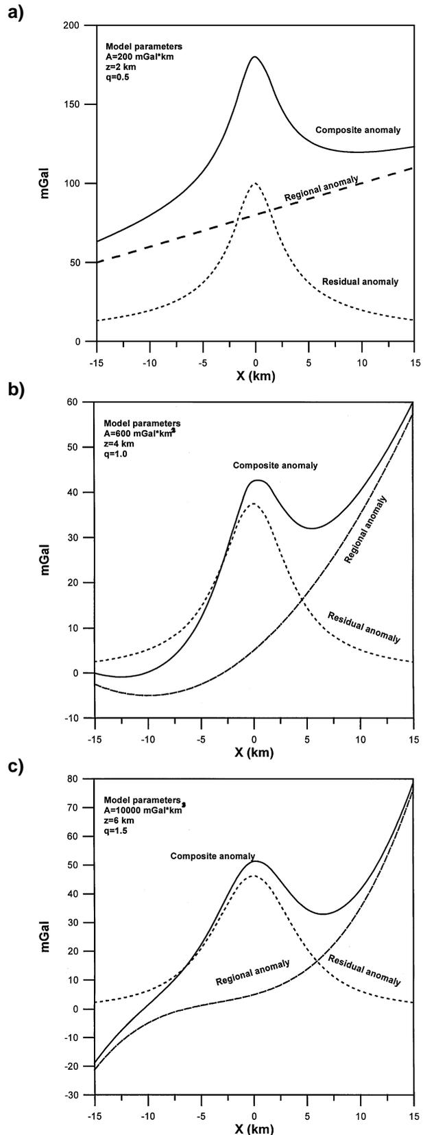
FIG. 1. Composite gravity anomaly (a)  $\Delta g_1$  of a buried vertical cylinder and first-order regional anomaly as obtained from equation (8), (b)  $\Delta g_2$  from equation (9), and (c)  $\Delta g_3$  from equation (10).
