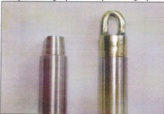
Fig 1: Left: A standard stainless steel model of a standard complete crown preparation. Right: A well-fitting cast crown seated on the stainless steel model with a loop for testing the tensile bond strength. Note the flat upper surface of the loop for application of seating force during cementation.
