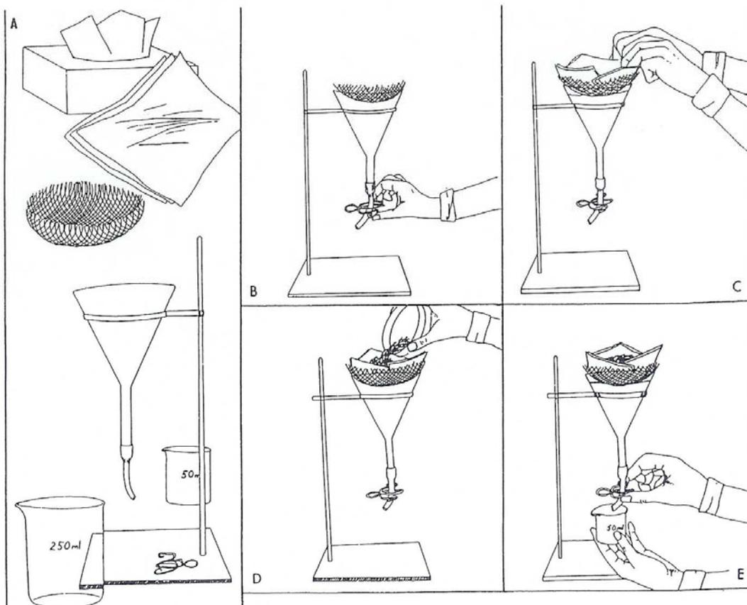
**Fig 3. Extraction nematodes from soil and plant materials by the Bearmann Funnel Technique.**
