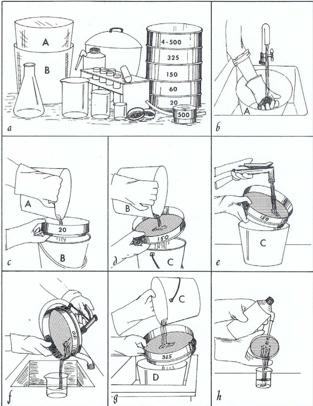
**Fig 4. Extracting nematodes from soil by Cobb's sieving gravity method.**
