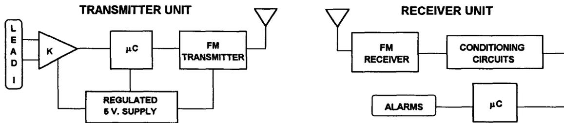
Figure 1: Block diagram of biotelemetry system
