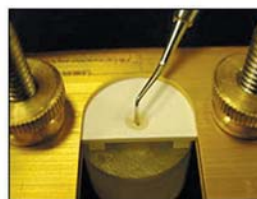
Figure 13. Generally, “unidose” capsules should be used to begin filling the insert mold.
