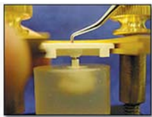
Figure 16. The clamp screws are carefully loosened. A condenser tip is used to gently hold the specimen in position as the insert is lifted up.
