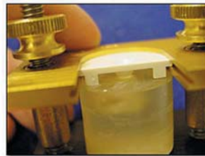
Figure 12. Great care must be taken when positioning and securing the polyethylene bonding mold insert so as not to damage the knife edge.
