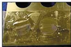
Figure 7. Transparent cellophane tape closes one end of the specimen mold and makes it possible to see the specimen to adjust the orientation of the specimen in the mold hole.
