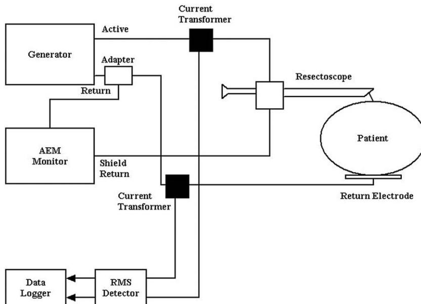
**Figure 1** Diagrammatic representation of instruments and circuitry.
