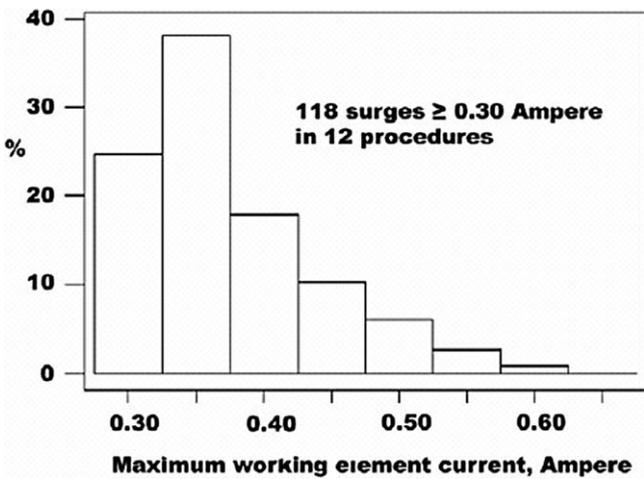
**Figure 6** Histogram of the amplitude of the peak surge currents.
