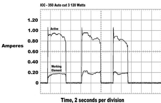
**Figure 3** Baseline active and working element currents.
