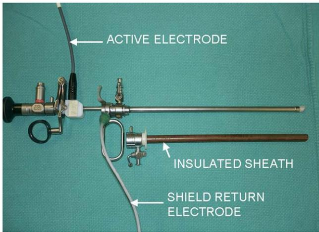
**Figure 2** The internal conductive components of the working element are electrically connected to the Encision Active Electrode Monitoring protection circuitry. The outer sheath has been changed to a nonconductive material to eliminate the concern that the active currents could be collected via the outer conductive sheath to the electro-surgical unit (patents pending).
