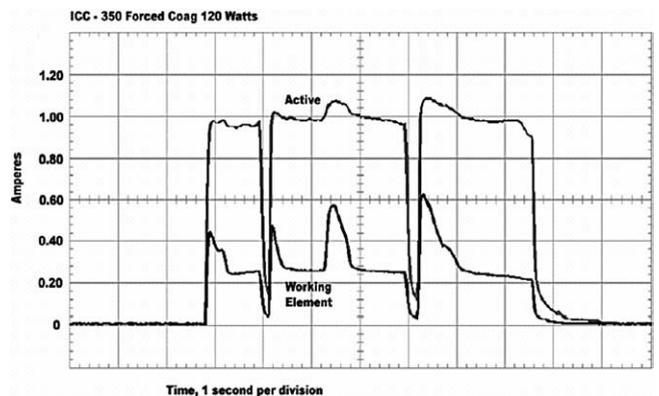
**Figure 5** Surge active and working element current with coagulation waveform.
