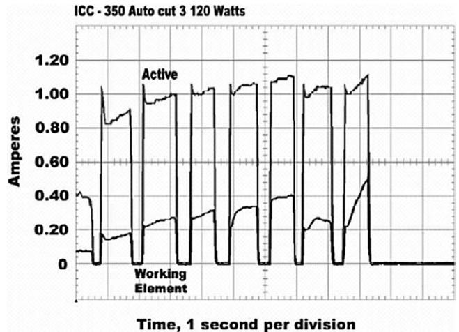
**Figure 4** Surge active and working element currents with cut waveform.
