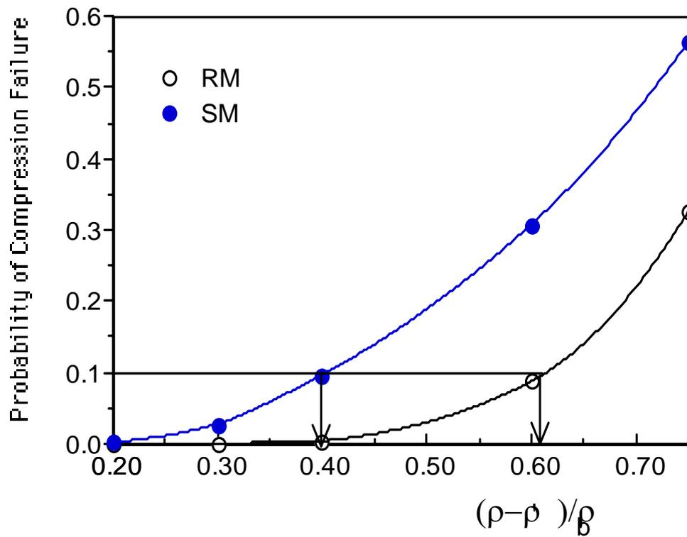
Fig. 3 Variation of the Probability of Compress Failure with Reinforcement Ratio
