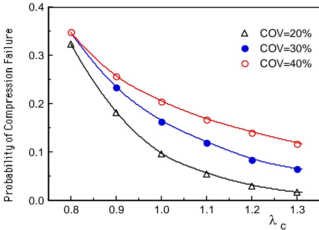
Fig. 2 Variation of the Probability of Brittle Failure with the Mean-to-Nominal Ratio of Compressive Strength of Concrete
