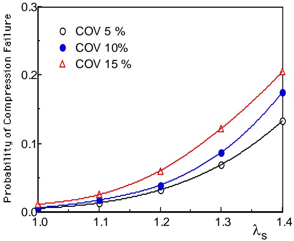
Fig. 1 Variation of the Probability of Compression Failure with Yield Strength of Steel
