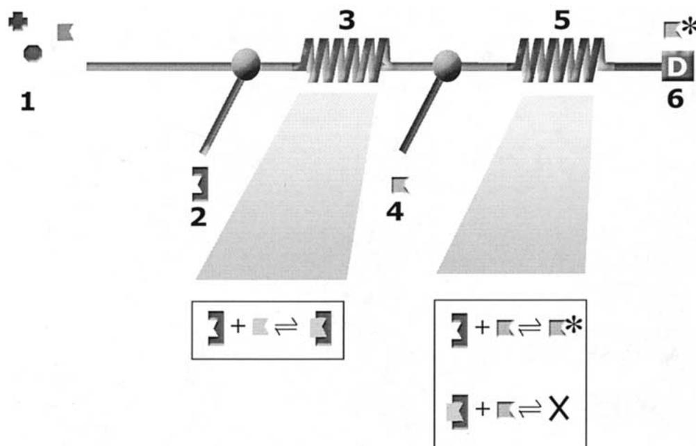
Figure 3. Schematic representation of a substrate conversion based bioassay format. 1. Injection of analytes. 2. Addition of enzyme. 3. Reaction coil. 4. Addition of internally quenched substrate. 5. Reaction coil. 6. Fluorescence detector.
