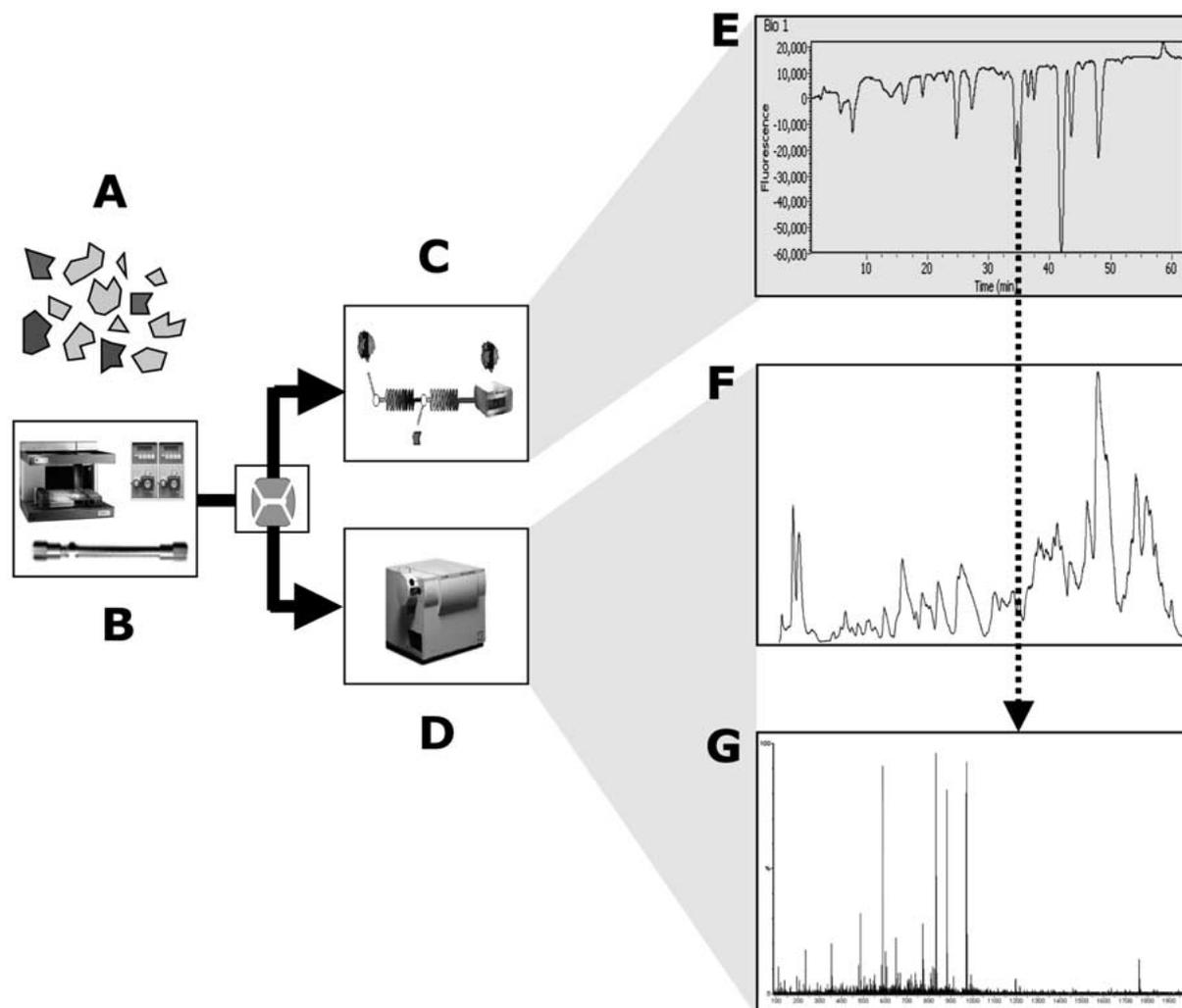
**Figure 1.** Schematic representation of on-line liquid chromatography – biochemical detection coupled to mass spectrometry. A. Injection of complex mixture. B. Separation of mixture by HPLC. C. Analysis of mixture by continuous-flow biochemical detection. D. Analysis of mixture by mass spectrometry. E. Output biochemical detection: bioaffinity chromatogram. F. Total ion current MS (TIC). G. Mass spectrum corresponding to response indicated in the bioaffinity chromatogram.
