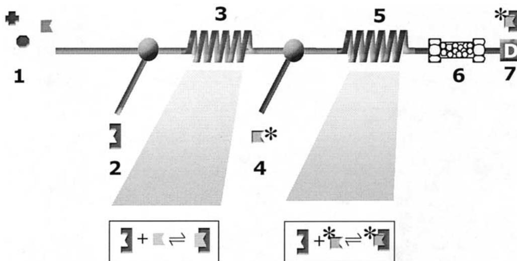
Figure 2. Schematic representation of a competitive bioassay format. 1. Injection of analytes. 2. Addition of cathepsin D (100 nM, 10  $\mu$ l/min). 3. Reaction coil. 4. Addition of pepstatin-BODIPY FL (10 nM, 10  $\mu$ l/min). 5. Reaction coil. 6. Restricted access column (ADS, C18, 2 \* 5 mm). 7. Fluorescence detector.
