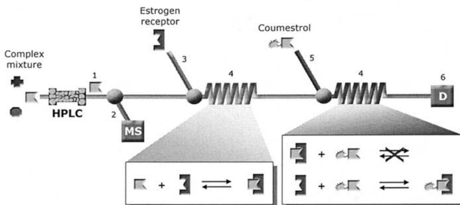
Figure 4. (A) Scheme of the FlowScreening configuration. 1. Autoinjector used for sample handling and selection. Injection into carrier solution; 2. Addition of coumestrol solution; 3. Reaction coil; 4. Fluorescence detector (D).
