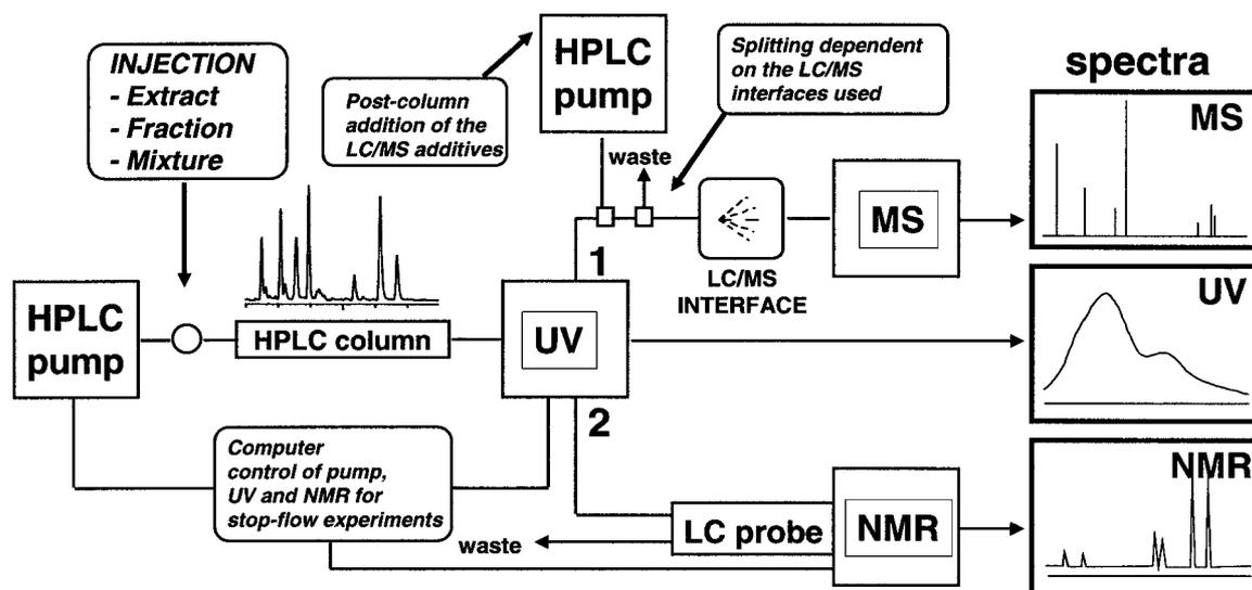
Figure 4. Equipment for LC/UV/MS and LC/UV/NMR analyses of plant extracts.
