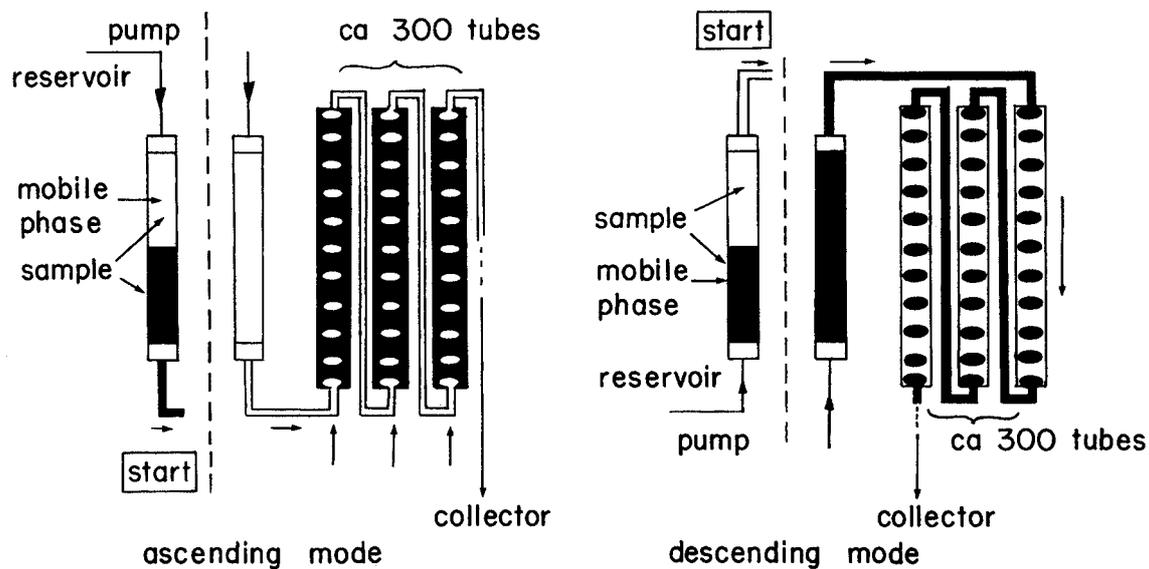
Figure 2. Droplet countercurrent chromatography.
