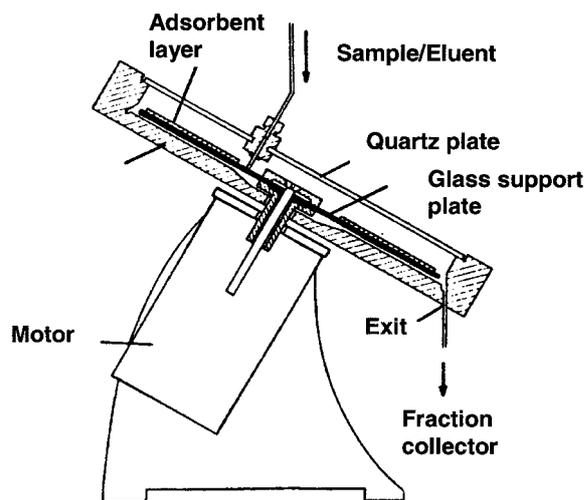
Figure 1. The Chromatotron CTLC instrument.
