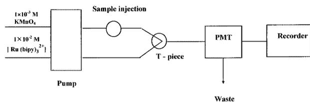
Fig. 1 Flow-injection manifold for CL determination of enalapril maleate.
