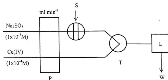
Fig. 2. FI manifold for the chemiluminescent determination of the substituted benzamides: p, peristaltic pump; S, sample port; T, perspex T-piece; L, luminometer; W, waste.
