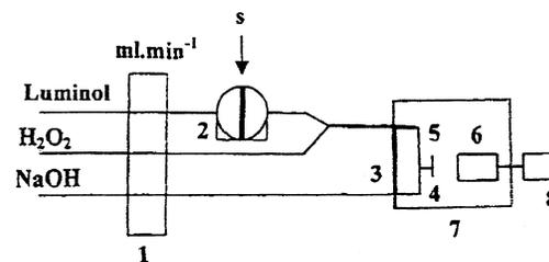
Fig. 1. Flow-injection manifold used for the CL determination of potassium clavulanate and sulbactam sodium; (1) peristaltic pump; (2) sample injection; (3) Perspex T-piece; (4) waste; (5) coiled flow cell; (6) photomultiplier tube (PMT); (7) housing; (8) recorder.
