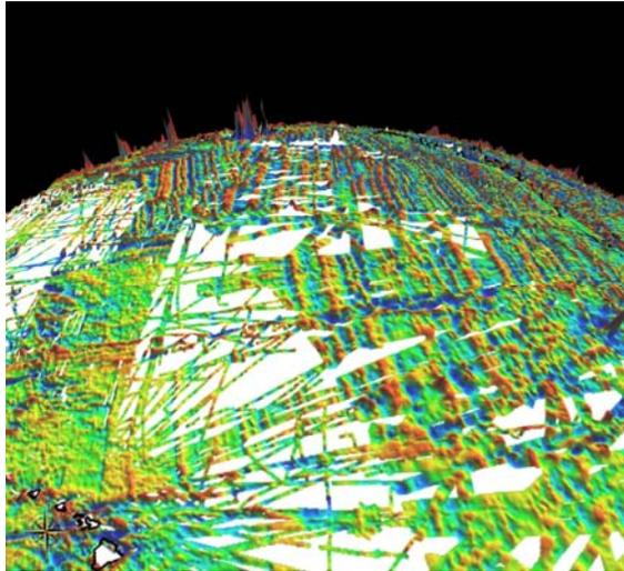
Figure 2: Our global magnetic anomaly grid in the 3D display software *NASA World Wind*. Shown here is a view northward from Hawaii. The *World Wind* plug-in can be downloaded from:
