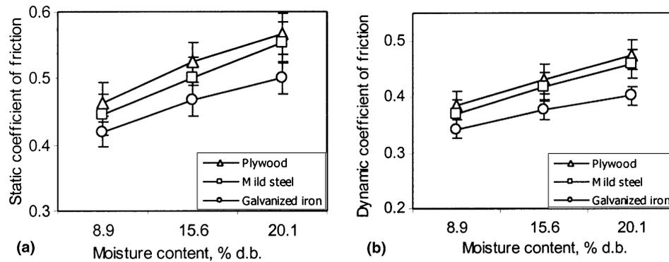
Fig. 6. Effect of moisture content on static and dynamic coefficient friction of fenugreek seeds against various surfaces: plywood, mild steel, galvanized metal.
