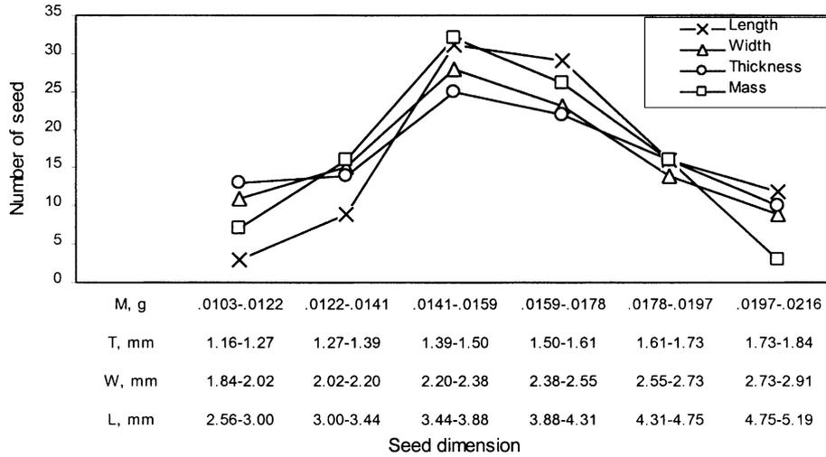
Fig. 1. Frequency distribution curves of fenugreek seed length, width, thickness and unit mass of the seed at 8.9% moisture content (db).
