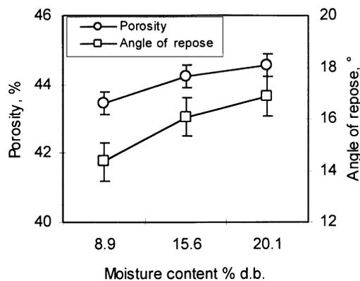
Fig. 5. Effect of moisture content on porosity and angle of repose.
