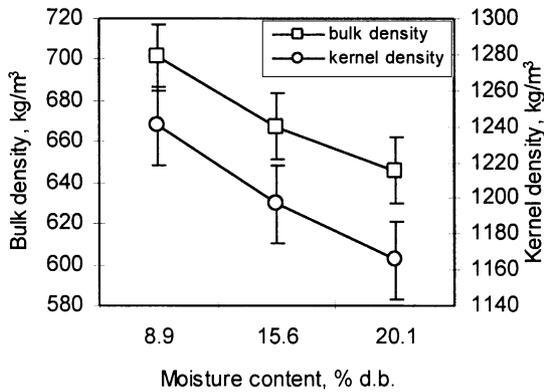
Fig. 4. Effect of moisture content on bulk density and kernel density.
