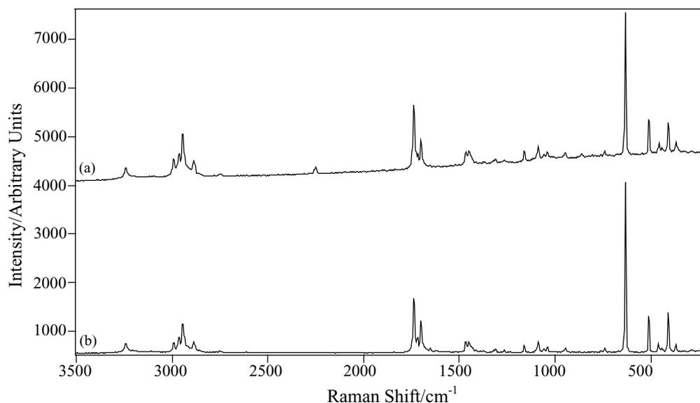
Fig. 3. Raman spectra obtained from (a) crystal in cyanoacrylate-fumed barbital-doped fingerprint and (b) barbital crystal.
