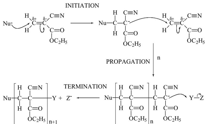
Fig. 1. Anionic polymerisation mechanism of ethyl-2-cyanoacrylate.
