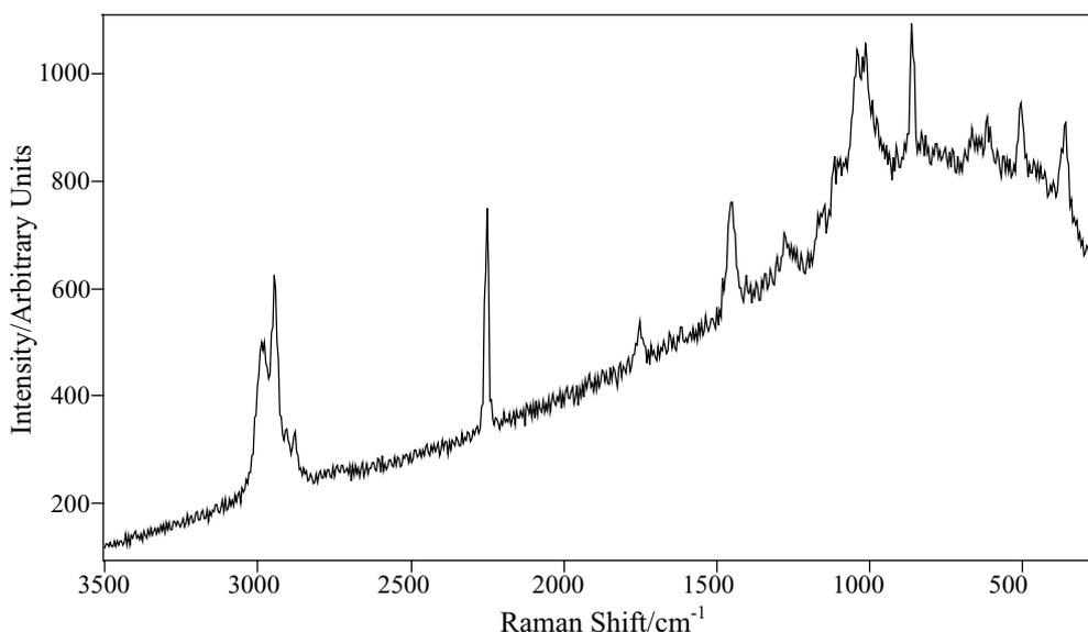
Fig. 2. Raman spectrum obtained from polymer-covered area of a cyanoacrylate-fumed fingerprint (after 10 min photobleaching).
