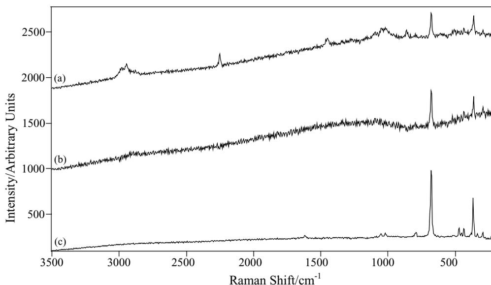
Fig. 5. Raman spectra obtained from (a) crystal in cyanoacrylate-fumed talc-doped fingerprint (after 40 min photobleaching); (b) same spectrum after subtraction of spectrum of cyanoacrylate polymer; and (c) talc crystal (after 15 min photobleaching).
