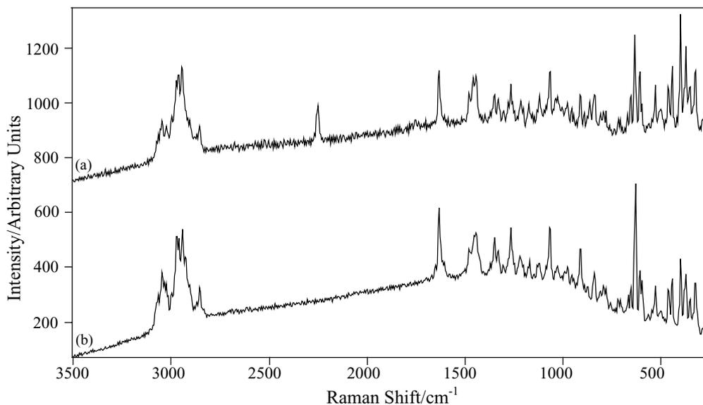
Fig. 4. Raman spectra obtained from (a) crystal in cyanoacrylate-fumed codeine phosphate-doped fingerprint and (b) codeine phosphate crystal (after 30 min photobleaching).
