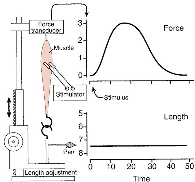
**FIGURE 9.7** A simple apparatus for recording isometric contractions. The length of the muscle (marked on the graph by the pen attached near its lower end) is adjustable at rest but is held constant during contraction. The force transducer provides a record of the isometric force response to a single stimulus at a fixed length (isometric by definition). (Force, length, and time units are arbitrary.)
