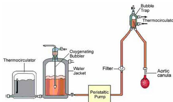
**Figure 1.** Illustration of the Langendorff System. The water jacket contains the perfusate fluid that is heated by the thermocirculator and oxygenated through the oxygenator bubbler. The perfusate is pumped by a peristaltic pump, then passes through a filter to the bubble trap where perfusate (also connected to the thermocirculator to maintain constant temperature) perfuse the heart via the aortic cannula.
