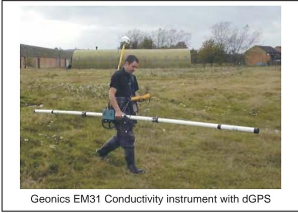
Buried foundations and other manmade structures can be an expensive obstacle in land reclamation schemes. TerraDat routinely carries out geophysical reconnaissance surveys to identify buried structures and other subsurface hazards for reclamation or remediation of brownfield sites. This information may then be used by the Client to optimize a trial pitting or borehole program with minimized risks.
