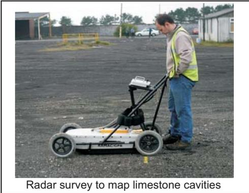
Ground penetrating radar (GPR) utilises pulsed high frequency radio waves to probe the subsurface without disturbing the ground. The GPR data are collected continuously as the instrument is towed over the ground surface and provides a real-time graphic image of the subsurface.
